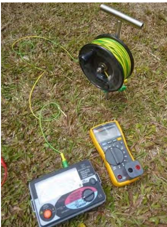
Example of a proprietary "independent earth" test unit
